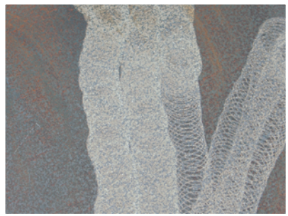
Water Blasting With Rotating Nozzles.
