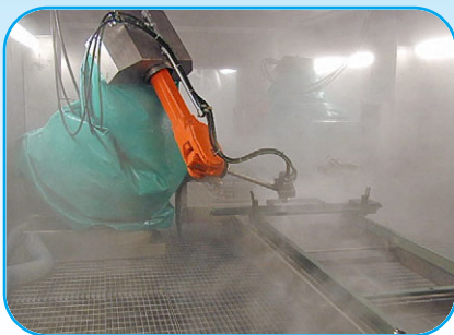
Robotic cleaning of skids at automotive plant. 100 lpm / 1000 bar
